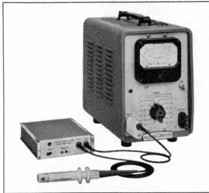
Fig. 13. -hp- Model 456A Current probe as used with -hp- Model 400D VTVM.
